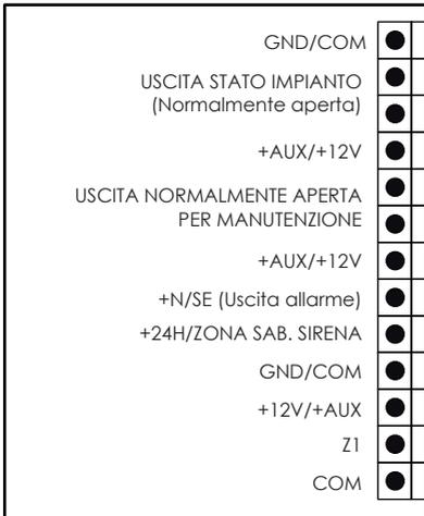
**SIRANDER LITIO (cod. 900126) COLLEGAMENTO CON USCITA ALLARME ANTISCHIUMA
