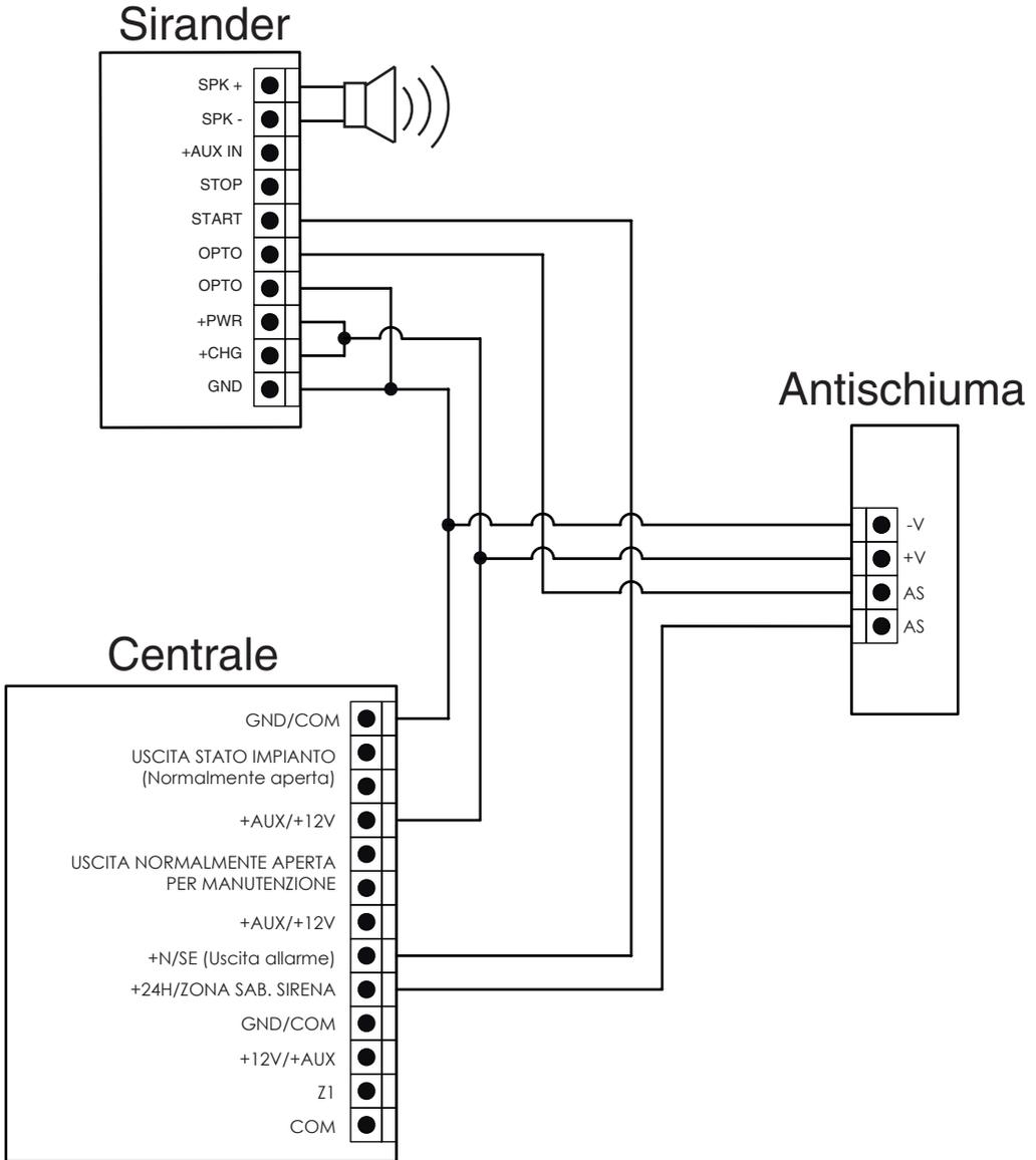
**SIRANDER LITIO (cod. 900126) COLLEGAMENTO CON USCITA ALLARME
